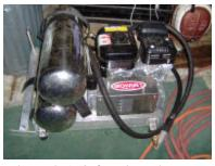
4 divers at once through 150-foot long hoses. This type of air delivery allows divers more freedom to work and provides an unlimited supply of air.
